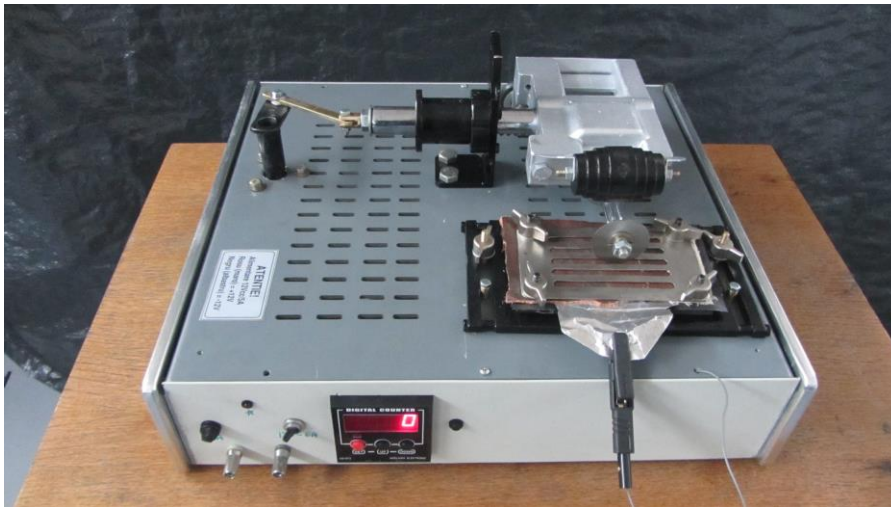
Fig.3. Test stand for determination of blade cut resistance of protective gloves
