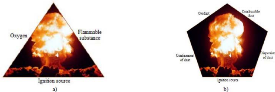
Fig.1. a) explosion triangle (for gases, vapours, mists); b) explosion pentagon (for dusts, lint and fibres)
